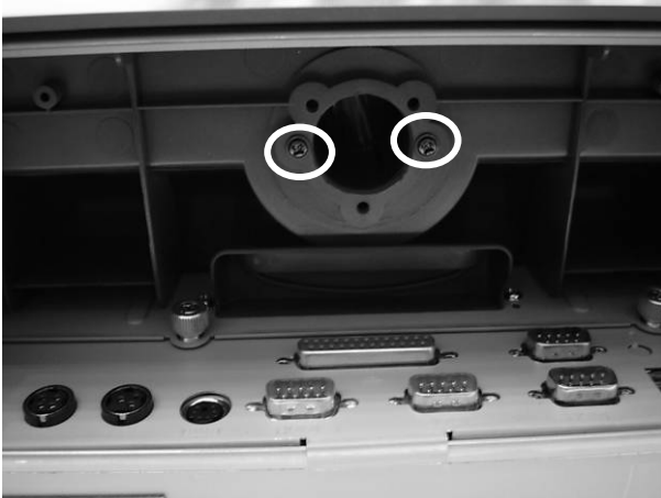
c. Tighten the screws (2) under the pole.
