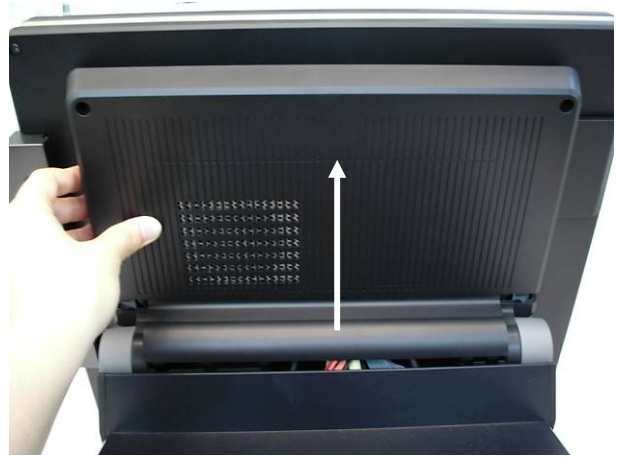
b. Lift the cover up and remove it.
