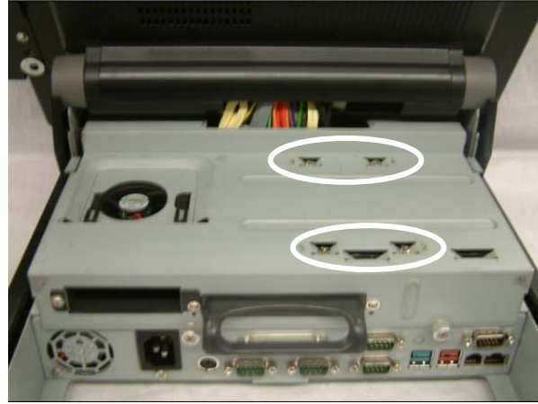
b. Remove the screws (4) to replace the HDD.
