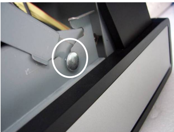
e. Fix the base cover in the open position as shown in the picture.
