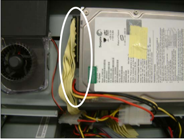
a. Disconnect the IDE cable (1) and power cable (1).
