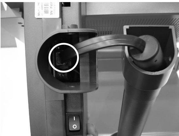
e. Connect the cable into the display.
