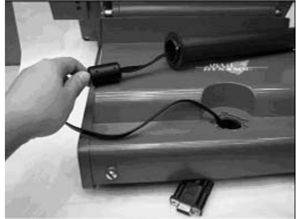
b. Pass the cable through the pole. Place the short or long pole into the hole.
