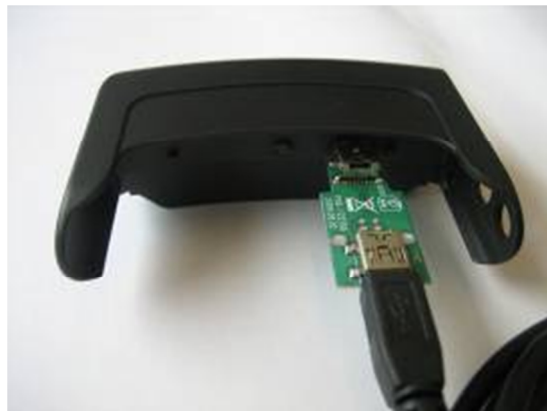
The custom cable connects to WF35 MSR & PC.
