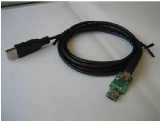
Custom USB cable (mini-USB cable + converter)
