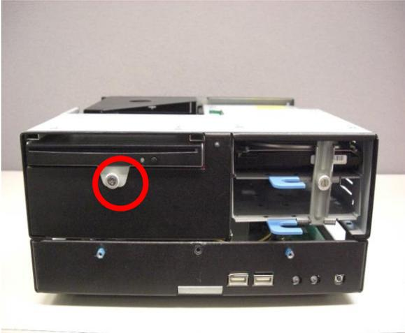
a. Loosen the thumb screw (1).
