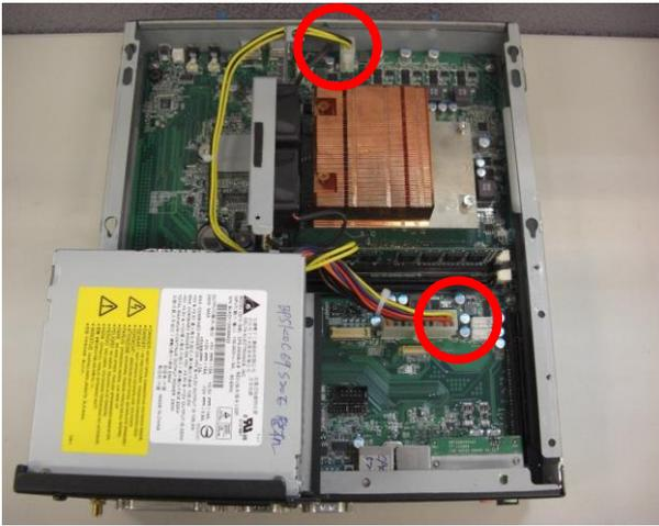
d. Disconnect the cable (2) of the power supply.
