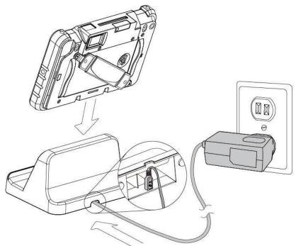
1. Connect the USB adapter to the connector on the bottom of the cradle charger and the power outlet.
