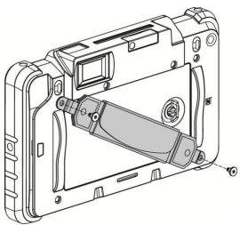
1. Attach the hand strap to the back of the system and fasten the screws (x2) to secure it.
