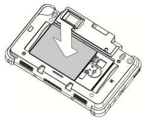
3. To install the battery put the battery in the slot and push until the battery clicks into place, put the batter cover back in and secure the pen screw clock-wise.
