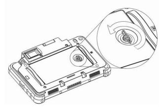
1. Loosen the pen screw counter-clockwise.
