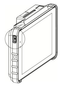
Push the power button to turn on the system and hold 4~6 seconds to turn off the system. Note: For the best touch performance, remove the protective plastic overlay from the LCD screen by peeling it away from one of the corners. Be sure to use a soft pointing device or finger tip to avoid scratching the screen during normal use.
