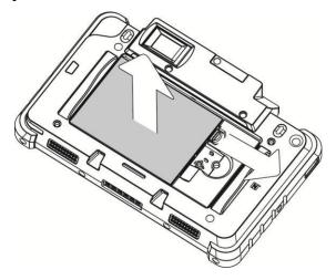
2. To remove the battery pull the plastic tab aside and gently pull the battery out.
