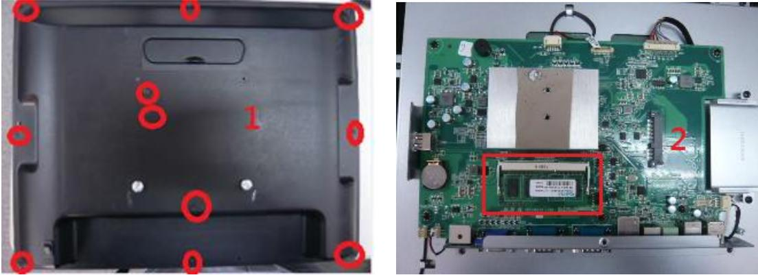
1. Loosen 11 screws and remove the back cover.
