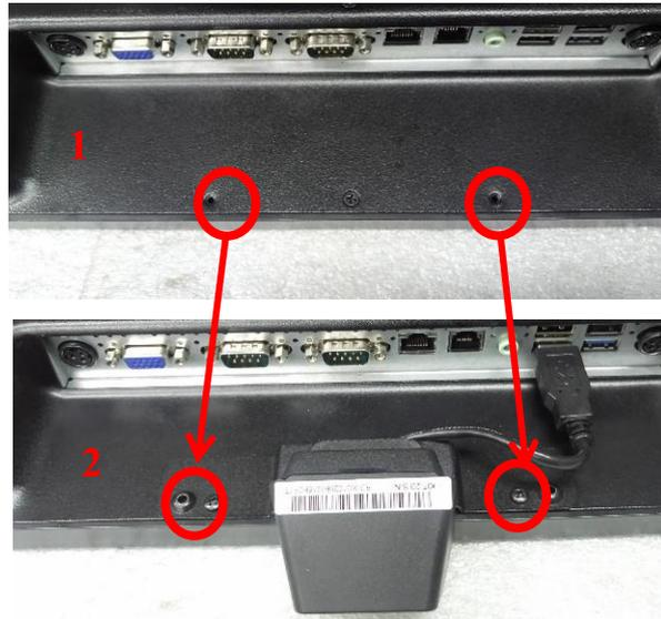
1. Install the barcode scanner with bracket attached by tightening the 2 screws
